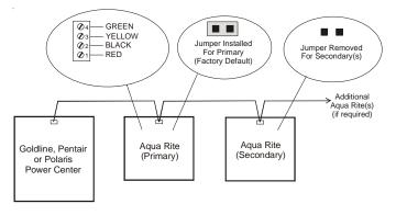
Goldline - Attach wires to proper screw terminals as shown below.
