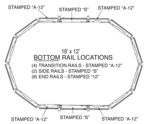
Place bottom rails stamped "S" between the side verticals. Place the bottom rails stamped "A-12" on the outside edge of the side supports as shown above. Place bottom rails stamped "12" on the ends of the pool.
