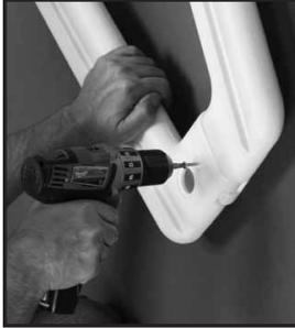
**#7:** Connect the top of the rails together using two #10 x 1-1/4" self-tapping screws (one in the designated mark on the inside rail and one on the outside rail).
