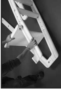
**#3:** Slide one tabbed end of the platform under the rails closest to the floor. Flexing the top rail downward slightly, slide the platform toward the top of the ladder until platform tabs fit into the locking holes in the rail.
