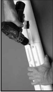
**#2:** Connect the Upper and Lower Outside Rails together using two #20 x 1/4" x 7/8" bolts and two 1/4 - 20 hex nuts. Repeat until all four rails are assembled.
