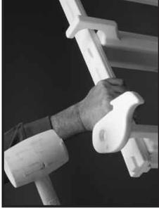
**#5:** Align the hole in the locking cam with the round tab on the locking slide tread and tap down. It may require several hits with rubber mallet. Repeat on the other side.
