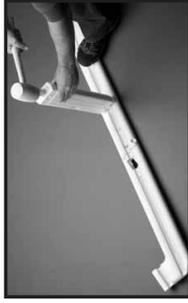
**#1:** Lay outside rail assembly on flat surface so that the notch in the hooked end is facing up. Insert tread into the opening second from the top and tap down.
