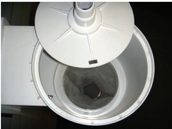
Vacuum Plate going onto Filter Cartridge
